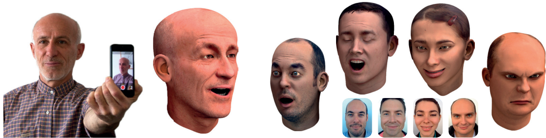
Figure 2.1 – Our system creates a fully rigged 3D avatar of the user from uncalibrated video input acquired with a cell-phone camera. The blendshape models of the reconstructed avatars are augmented with textures and dynamic detail maps, and can be animated in realtime.
