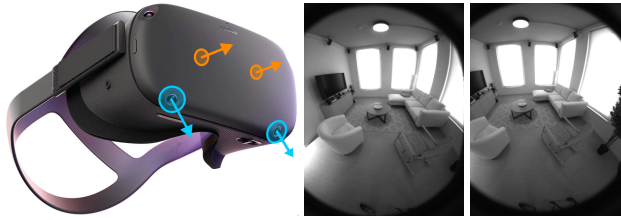
Fig. 2. Oculus Quest headset showing the position and orientation of cameras (blue) and the user’s viewing direction (orange), and example images from the bottom two cameras. Due to the optical distortion and the positioning of the cameras vs. the user’s eye positions, displaying the camera feed directly causes visual discomfort and motion sickness.
