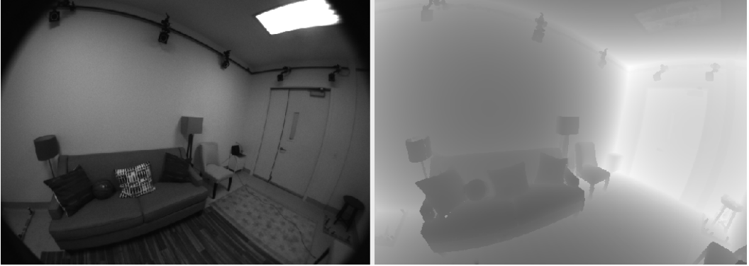
Fig. 8. Datasets. Input view (left) and corresponding pseudo ground truth depth map from a laser scan (right).
