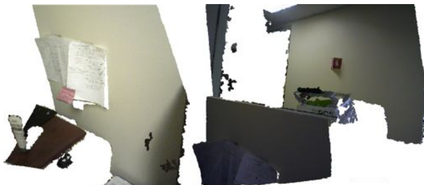
Figure 1.1: Typical jumps in the exposure settings of RGB-D cameras - the color of the wall changes from white to pitch black in just a few frames.
