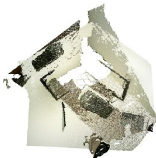
Figure 5.12: Example where the planes RANSAC method fails, as there are three ways in which the two frames representing one corner of a room can be aligned, and they cannot be discriminated by using just planes.
