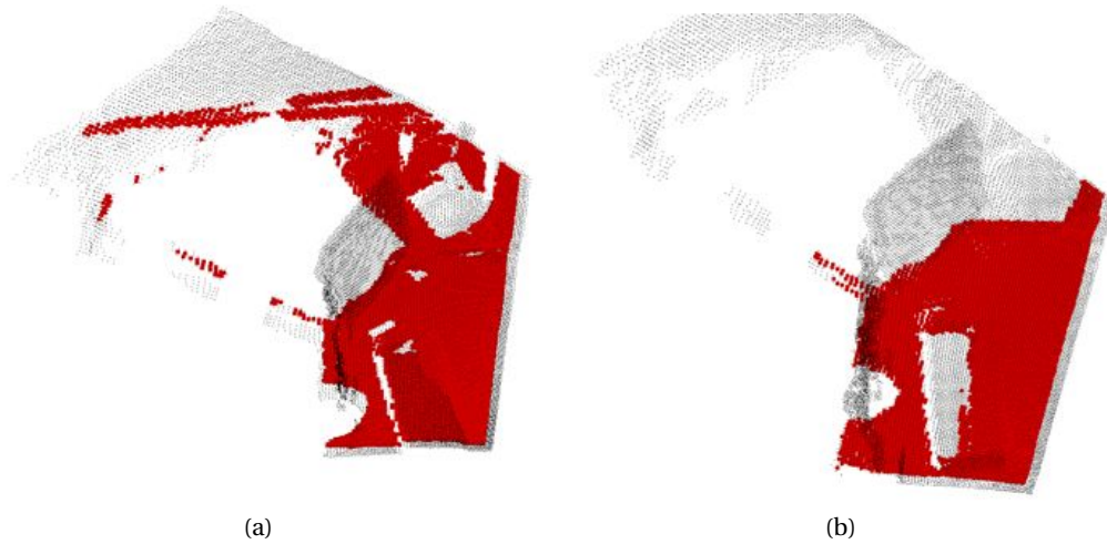
Figure 5.3: Clustering the planar inliers helps concentrate only on a single surface at a time. (a) Before clustering, raw output from the RANSAC plane fitting; (b) The largest cluster only.
