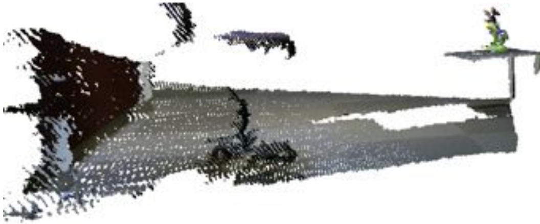
Figure 2.17: Example scene with a wider range of depths, that will be used to test the improvements brought by the weighting of the point pairs in the transformation estimation procedure.
