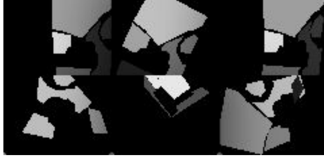
Figure 5.10: Example of the low resolution renderings used by the plane RANSAC algorithm for computing the number of inliers for a candidate source transformation.
